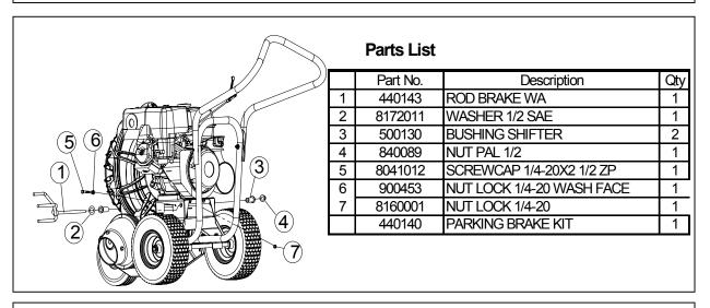
To apply parking brake, simply rotate forks to till they rest against the back end of the tire. Place once foot on top fork and gently put downward pressure on the fork while carefully pushing unit forward. The forward motion of the tire will help to roll the forks into a fixed position. To remove from braking position pull unit backwards rotating the tire, which will rotate the forks away from locked position on wheel.
